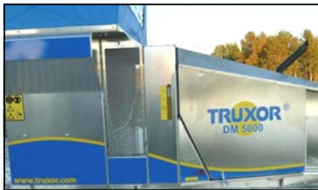
The air intake to the radiator has a filter that prevents insects, etc. from getting caught in the cells of the radiator.
