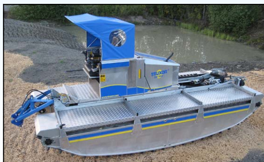
The movable driver's cab is hydraulically adjusted and works as a counter-weight during heavy lifts in water.
