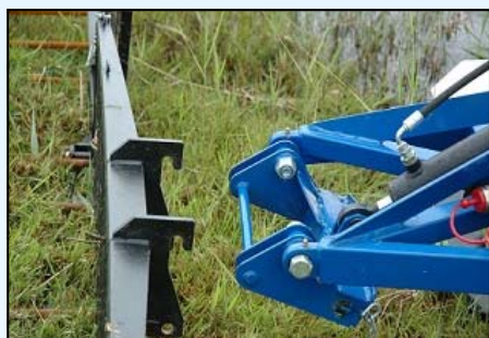
The DM-bracket allows for easy tool exchange.
